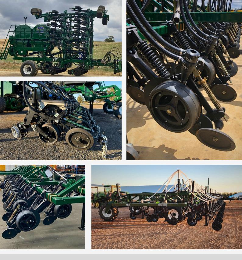
Excel Agriculture's row units are designed for durability, adaptability, and superior in-field performance. Whether single disc, double disc, or tyne configurations, our row units deliver the accuracy and reliability you need for optimal planting results.
